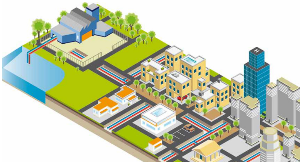
Figure 14: Illustration of a district cooling system (ref. /27/)
